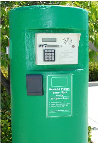
**Features** The DC-1023 reader contains a 2-color LED and a 4 kilohertz beeper. Both LED and beeper are controlled by the reader itself and also can be controlled externally by the host system. The LED can indicate access-granted by the host. The beeper can be used as an alarm that prevents further card reads until the alarm condition is cleared.
